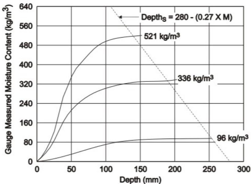
Figure 5. Effect of Moisture on Depth of Measurement
