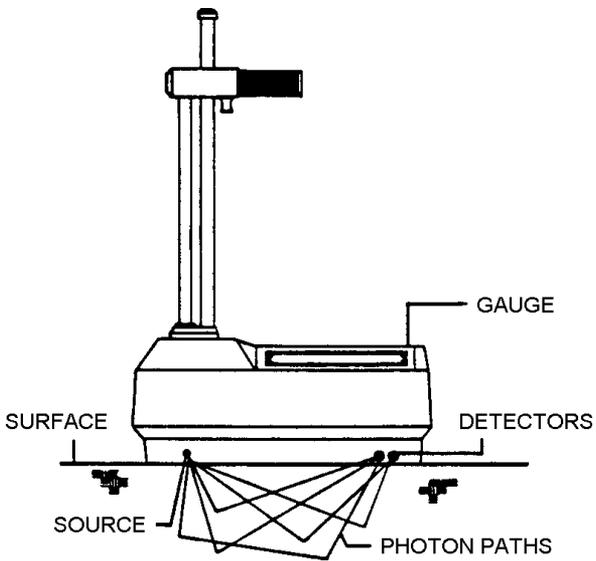
Figure 3. Backscatter Geometry
